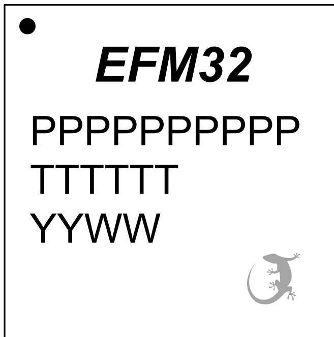
Figure 10.3. TQFP48 Package Marking
