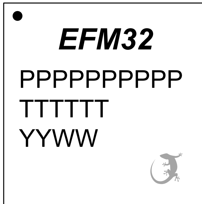
Figure 8.3. TQFP64 Package Marking
