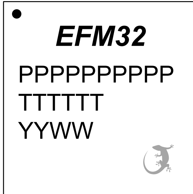
Figure 7.3. QFN80 Package Marking
